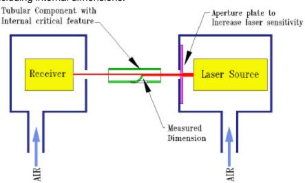
performs a Go/No-Go evaluation as the part passes by the measurement station. Low pressure air is used to keep the optics clean and part tracking is available to enable the rejection or sorting of non-compliant parts without stopping the process.
