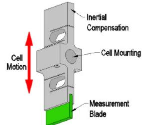
The system works by compressing, or deflecting the element to be tested with a load cell specifically designed for the purpose. The illustration is of a cell designed to measure the "rate" of spring or flexure components. The load cell is attached to an oscillating mechanism (possibly the forming press slide), and the SAM™ module captures the force information as the test piece is deflected. It can also be used for Insertion / withdrawal force measurements.
