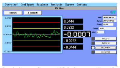
well as more simple controls which can track and reject specific parts which don't meet specific quality criteria.
