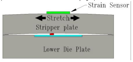
The system works by measuring the strain in the movable stripper plate. When a slug is present, the stripper plate will contact EARLY in the stroke, and "wrap itself" around the slug as shown in the exaggerated view below. This will cause an anomalous strain indication at a point in the stroke where normally nothing is occurring. Even if the slug embeds, the initial force signature will still be present, and signal the existence of the slug.
