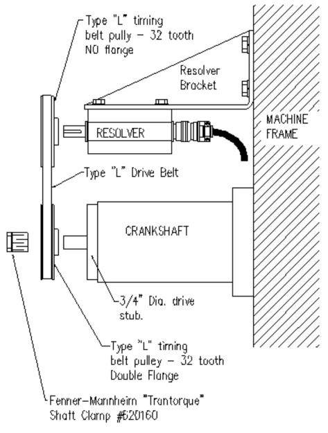
Figure #8 - Gear belt drive detail
