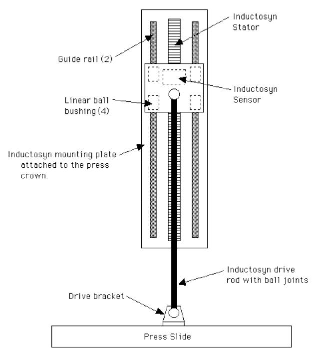
Figure # 11 - Typical Inductosyn<sup>TM</sup> installation
