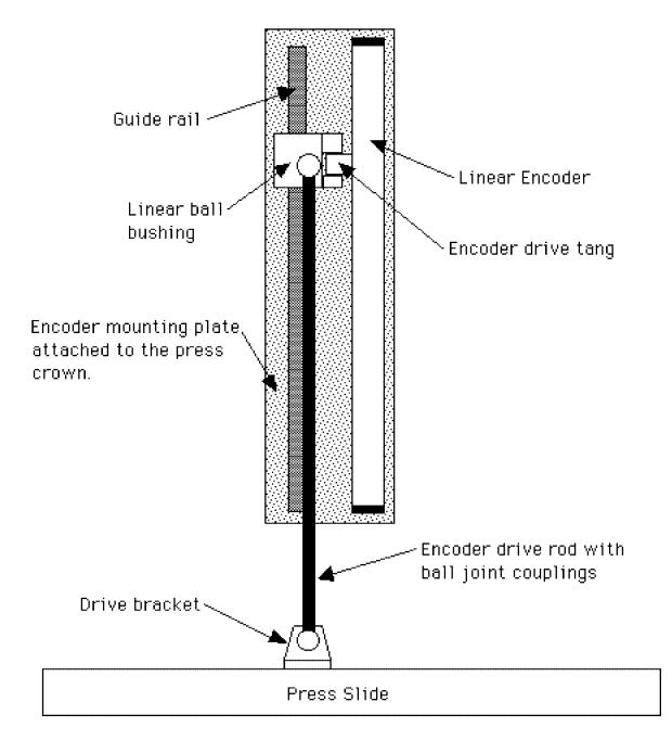
Figure # 10 - Linear encoder arrangement
