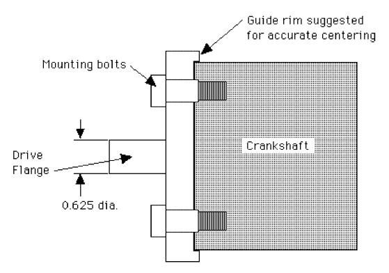
**Figure # 5 - Drive flange arrangement**
