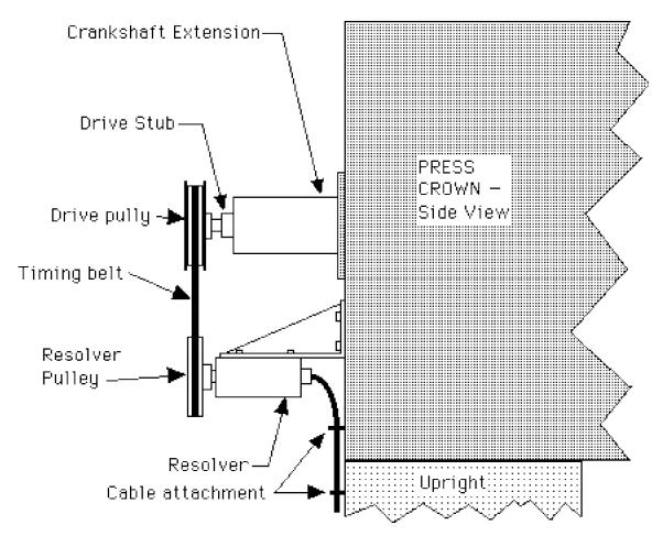
Figure #7 - General arrangement for a Timing Belt resolver drive
