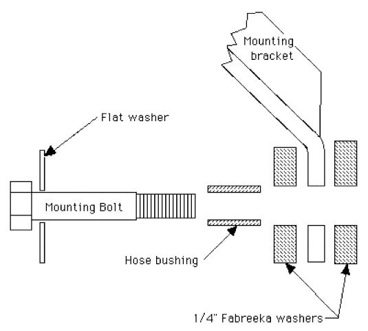
**Figure # 4 - Cushion mounts for Resolver bracketry**
