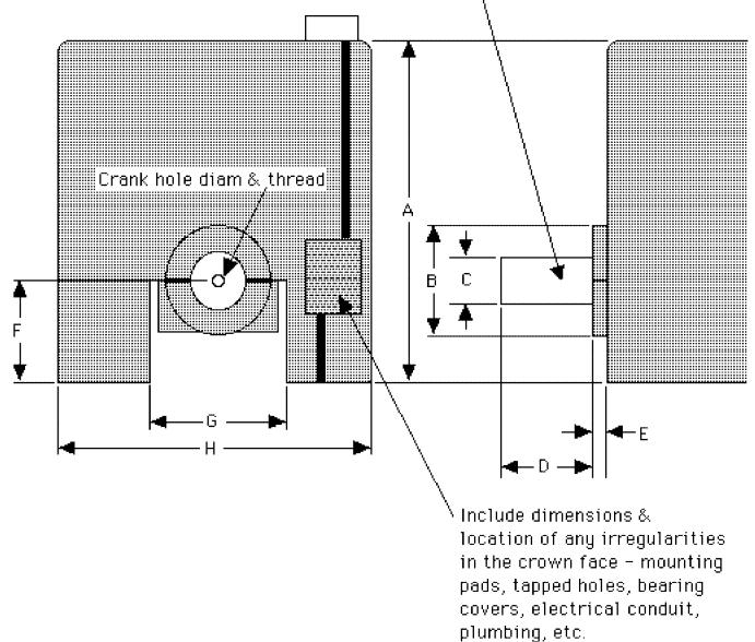
Figure #9 - Resolver mounting area dimension sketch
