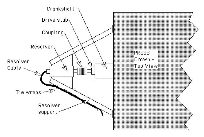
Figure #3 - Top view - Resolver end drive
