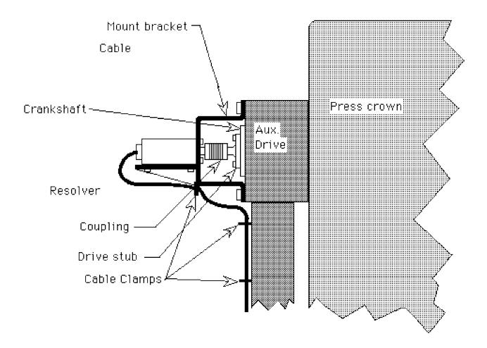
Figure # 6 - Auxiliary drive resolver mounting
