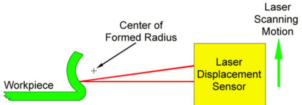
A high quality laser must be used because of the relatively severe angles encountered on the measured surface as shown. Differential measuring for “on the fly” measurement is also possible with multiple laser units. Post processing of the measured data also gives the ability to confirm that the radius is properly formed, and is a true radius. If the radius is true, then the center of the radius can be developed in both horizontal and vertical axes.
