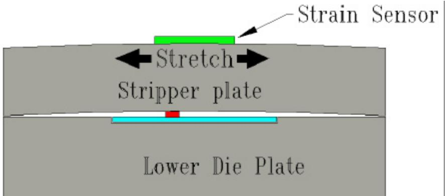
The system works by measuring the strain in the movable stripper plate. When a slug is present, the stripper plate will contact EARLY in the stroke, and “wrap itself” around the slug as shown in the exaggerated view below. This will cause an anomalous strain indication at a point in the stroke where normally nothing is occurring. Even if the slug embeds, the initial force signature will still be present, and signal the existence of the slug.
