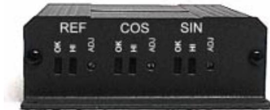
Figure # 9 - Indicators / Adjustments on the Resolver Converter.
