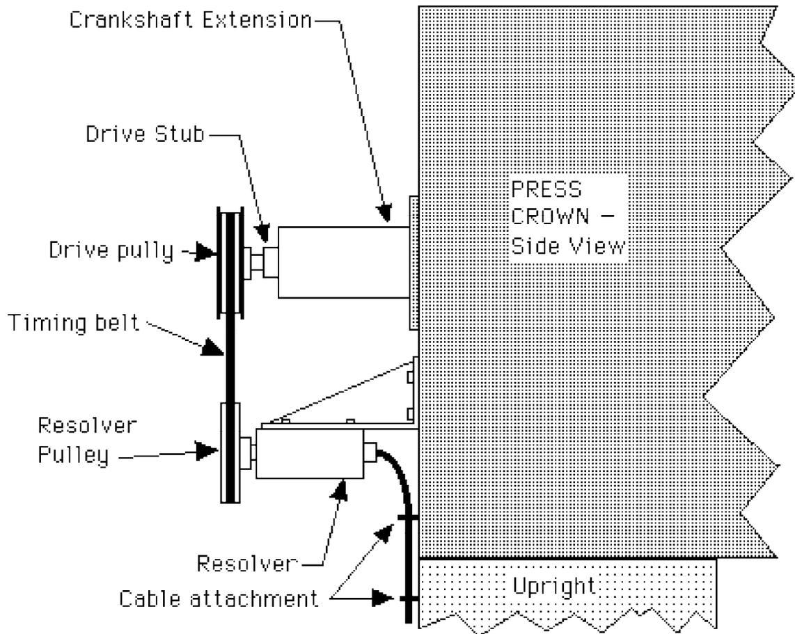
**Figure # 7 - General arrangement for a Timing Belt resolver drive**
