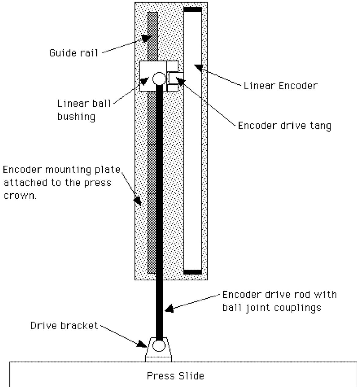
**Figure # 10 - Linear encoder arrangement**
