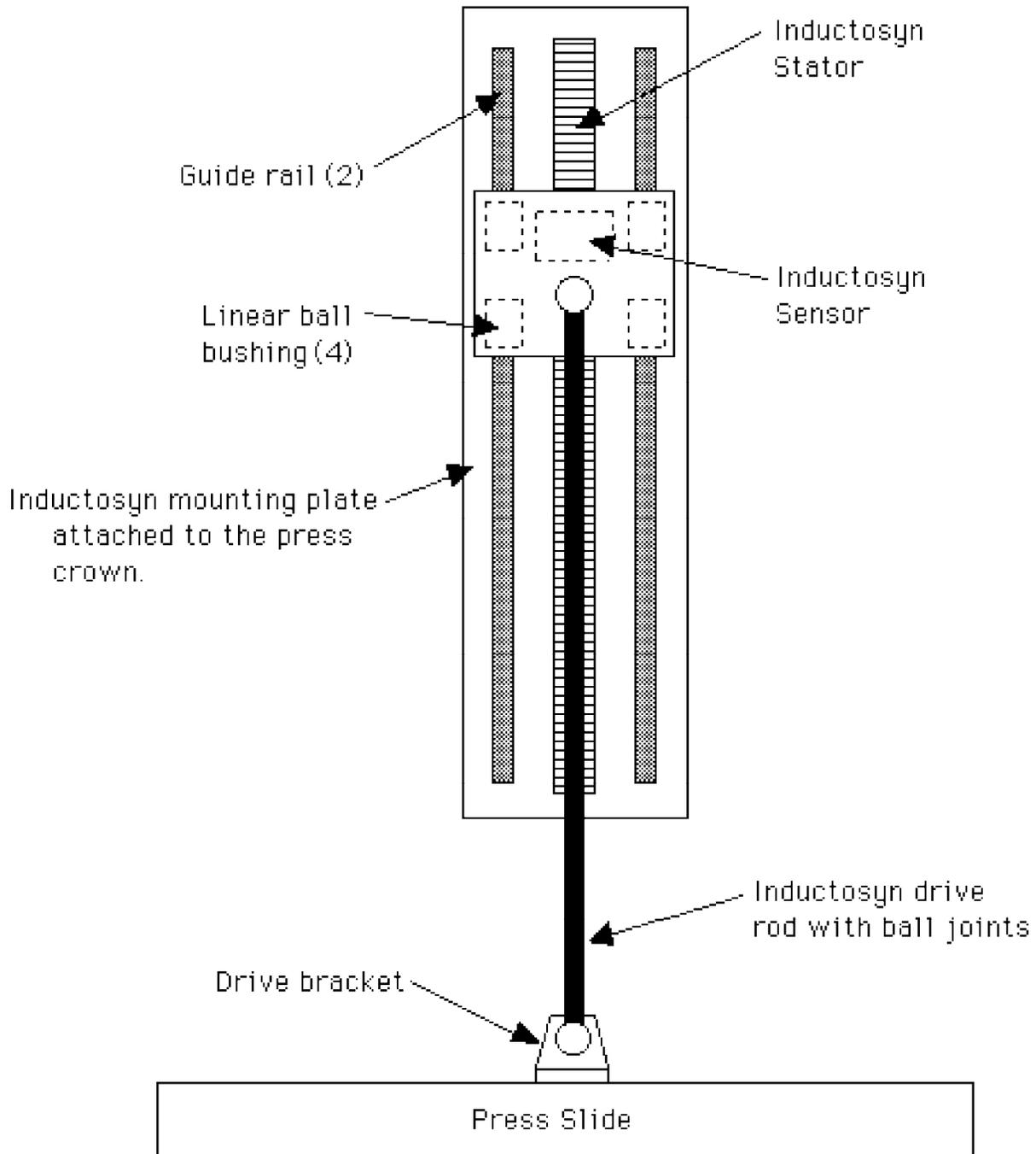
**Figure # 11 - Typical Inductosyn™ installation**
