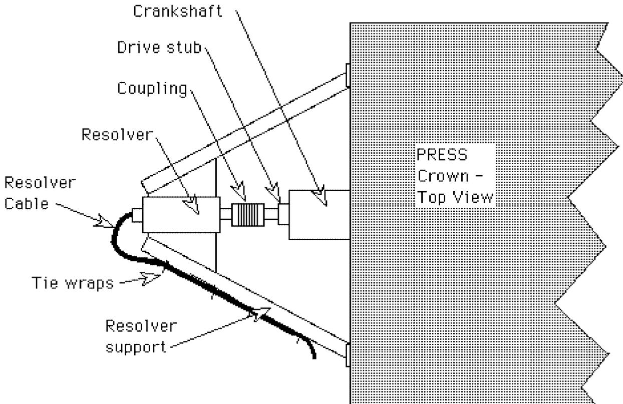
**Figure # 3 - Top view - Resolver end drive**
