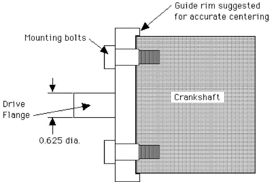
**Figure # 5 - Drive flange arrangement**
