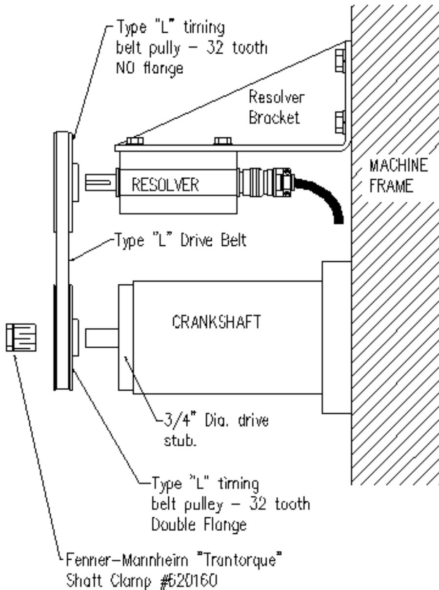
**Figure # 8 - Gear belt drive detail**
