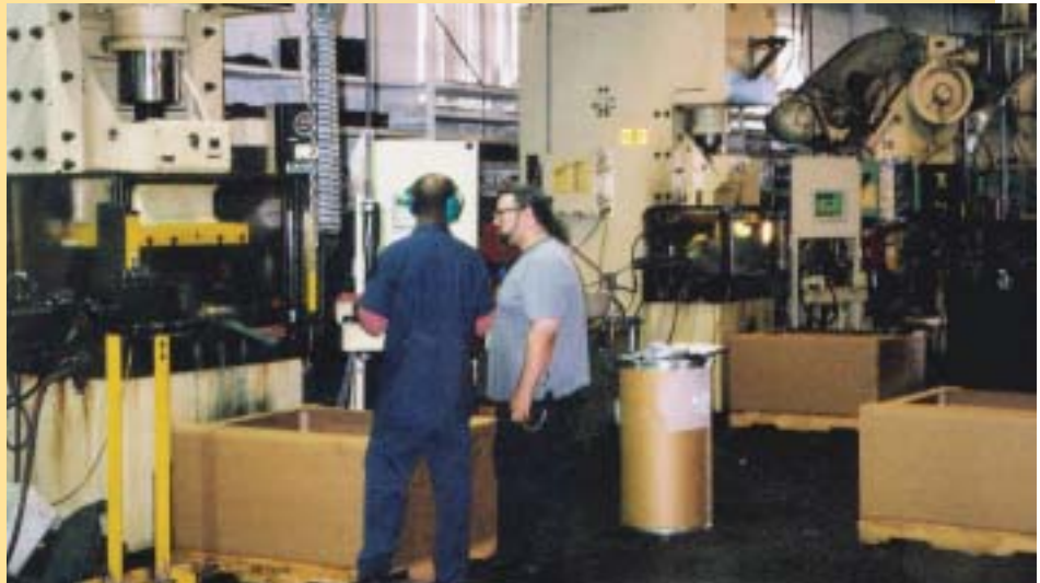
With controls and sensors in place, this operator can leave one press running unattended while he trains an employee on another.
